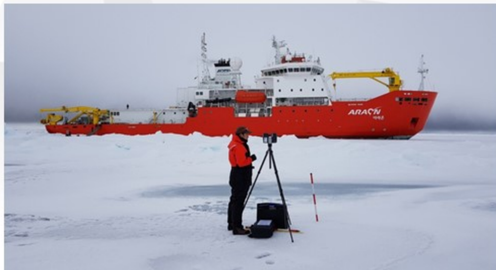
Ice surface roughness measurement using 3D scanner
