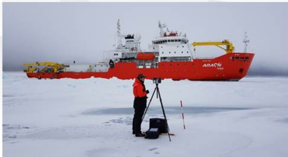
Ice surface roughness measurement using 3D scanner
