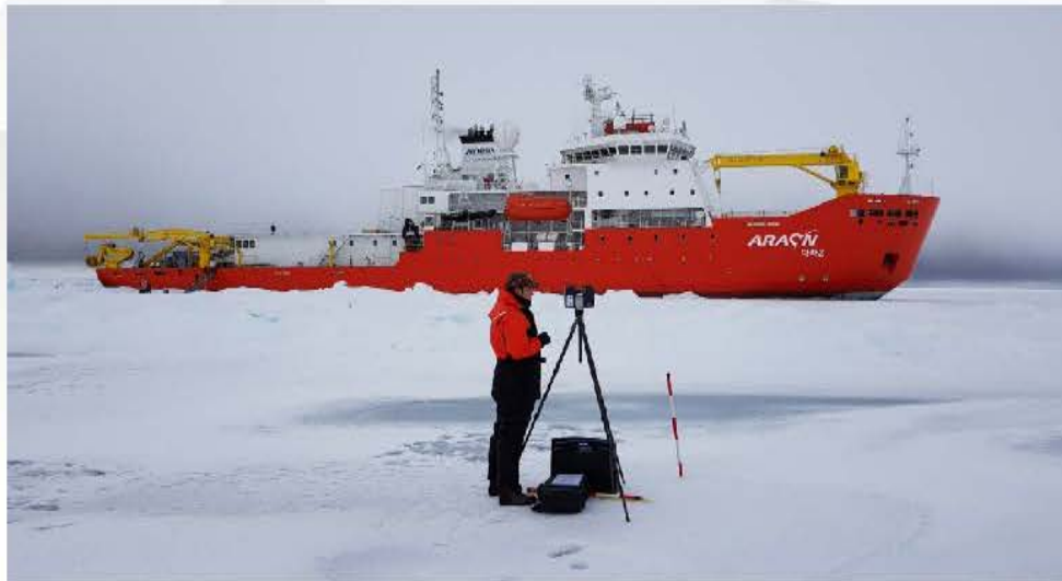
Ice surface roughness measurement using 3D scanner
