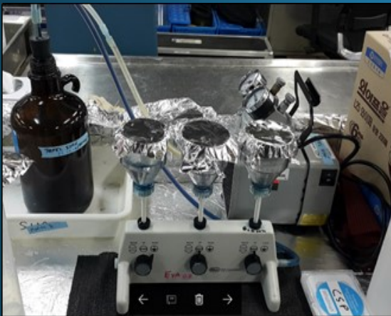
▲ Filtration systems for collecting TEP/CSP
