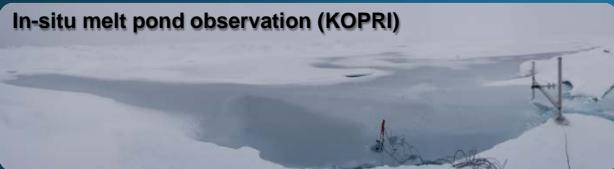
Melt pond Ice Mass Balance (IMB) with radiation sensors (KOPRI & BAS)
