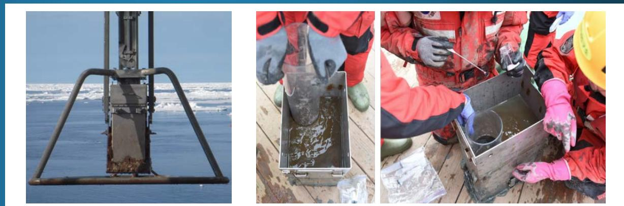
Box coring for recovery of undisturbed upper sediments
