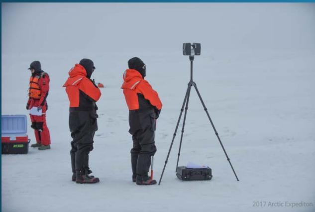
Ice surface roughness measurement using 3D scanner
