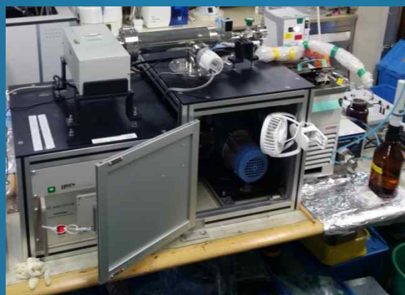
Membrane-Introduction Mass Spectrometry (MIMS) System for DMS measurement
