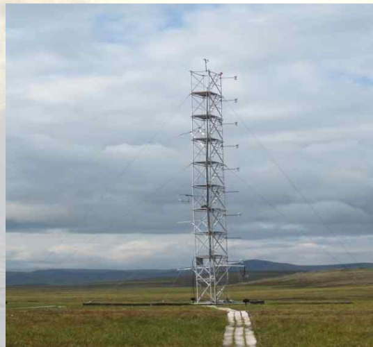
The tower for measurements of turbulent fluxes (the height 20 meters)
