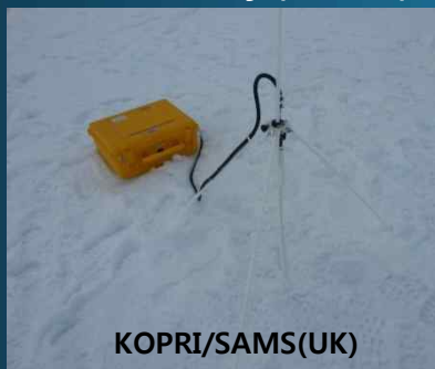
SAMS-type Ice Mass Balance Array (SIMBA)
