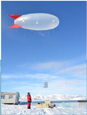
Tethered-zonde+Particle measuring instrument
