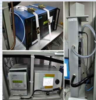
CRDS Shelter 02Deck (15m, Port) CRDS (G2301-f) Data logger (CR3000) Motion Sensor (MPII)
