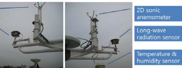
03Deck (38m) Net radiometer (PSP) Net radiometer (PIR) Temp & RH (HMP45D) Wind sensor (PTB100) Humidity sensor (LI-200) Data logger (CR3000) Anemometer
