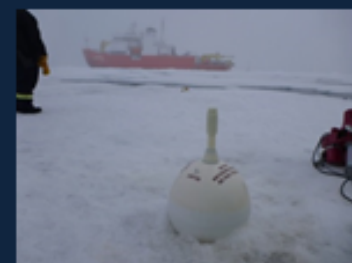
SATICE: High-precision GPS buoy (CSIC/MIT)
